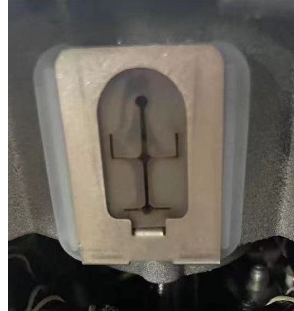
Clean and replaced flapper and flapper bracket
