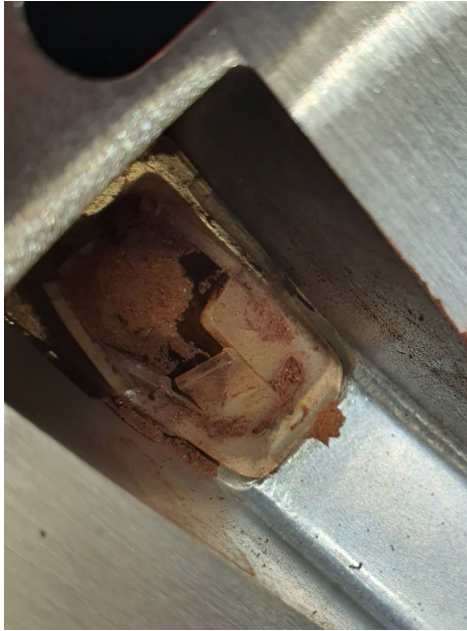
Deteriorated flapper and broken bracket
